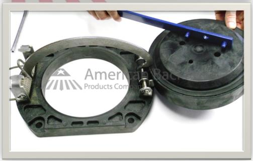
Using the retainer wrench, unscrew the disc retainer counterclockwise.
